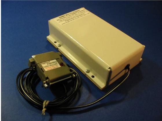
The *SWMA Memory Adapter* is designed to provide memory backup power for the Xantrex Trace™ SW and PS Series inverters. Without the *SWMA*, if both AC and DC (main battery) power is removed from the inverter the setup-menu memory is erased. With the *SWMA* the memory may be retained for up to two weeks. This allows the inverter system to be serviced without the need to reprogram the inverter's setup-menu parameters.
