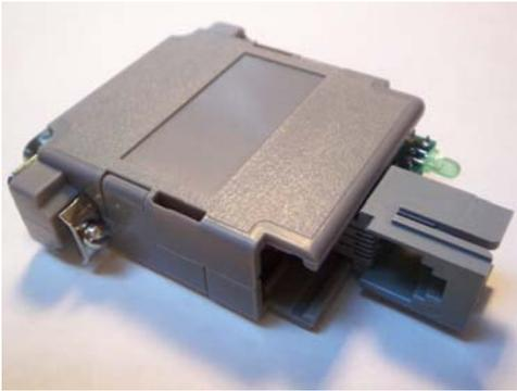
The *SWCA-II Communications Adapter* is designed to connect a Xantrex Trace™ SW-Series Inverter to a PC's RS-232 serial communications port. Although the *SWCA-II* is physically slightly different than the original Xantrex SWCA, it is electrically compatible in every way.
