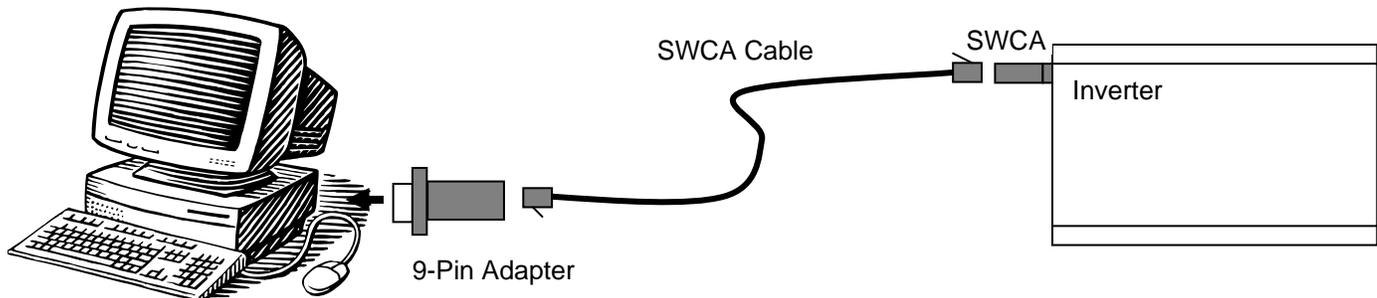
1. Begin by plugging the *SWCA-II* (pictured in the photograph) into the "Remote" port of the inverter. To avoid the possibility of changing the inverter's mode unintentionally as you plug it in, it is recommended to park your inverter's front panel display on the Meter's menu. The green LED on the back of the *SWCA-II* should illuminate when it is plugged in. It is normal for the LED to turn off by itself within 1 to 3 minutes if no PC software is communicating with the device.
