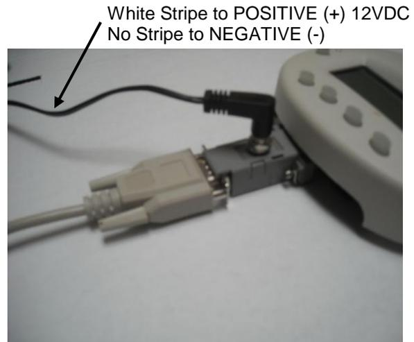
One possible source of 12 Volts DC is from an unused Aux Output of an OutBack inverter. Even if the battery bank feeding the OutBack equipment is 24 or 48 volts, the Aux Output can supply the needed 12 Volts DC. But the Aux Output must be configured to be the correct polarity, and must be configured to be steady (unchanging). Therefore, it can not be used for any other purpose.
