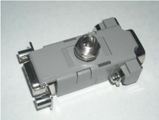
Because of the design of the OutBack Mate, certain types of serial port devices will not reliably work when plugged into the Mate's RS-232 port. The Mate's serial port is optically isolated to improve protection of circuitry, but this requires that the RS-232 signals to the Mate be of full strength, and be of the right polarity.
