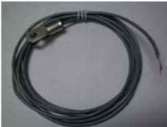
Most batteries loose capacity when they are cold. The addition of the temperature sensor allows your meter to compensate the battery's capacity (in Ampere-Hours, or Watt-Hours) using knowledge of the battery's temperature. The sensor has a 3/8" hole for mounting to a battery terminal.
