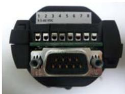
Formerly available only on the Link-10 "Choice" model, RHE can retrofit most Link-10s to add a 9-pin RS-232 serial communications port to allow interfacing to computers and other external data monitoring equipment.
