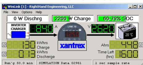
RHE's *WinLink* PC software runs under Windows 98 through Vista and provides real-time display and data logging of data provided by the Link-10 (meter serial port required). See our separate *WinLink* spec sheet for more details.
