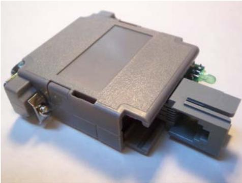
The *ICA-II Communications Adapter* is designed to connect a Xantrex Trace™ SW Plus-Series Inverter to a PC's RS-232 serial communications port. Although the *ICA-II* is physically slightly different than the original Xantrex ICA, it is electrically compatible in every way.
